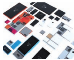
Ara will have a basic endoskeleton called the Endo that will hold the interchangeable components together through electro-permanent magnets
